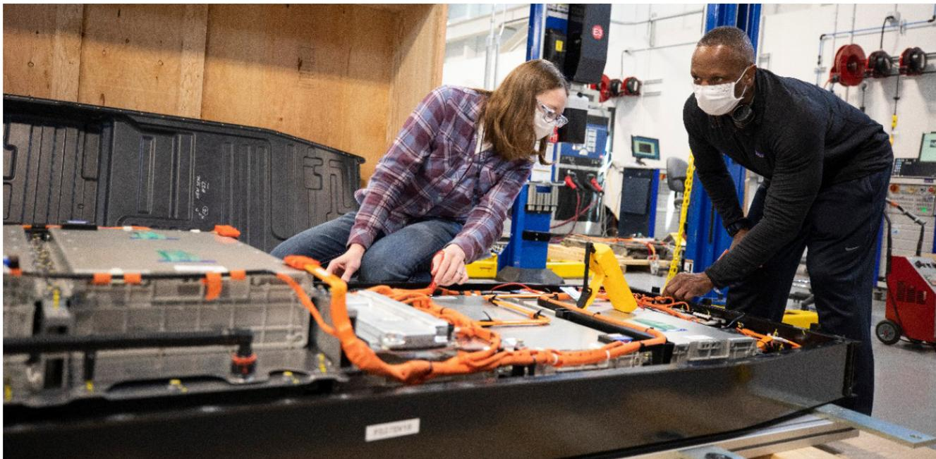
Dane Hardware, Ford Motor Co. design and release engineer, and Mary Fredrick, Ford Motor Co. battery validation engineer, examine internal components like cell arrays, wiring and contactor switches at Ford’s Battery Benchmarking and Test Laboratory in Allen Park, Michigan. Source: Ford
